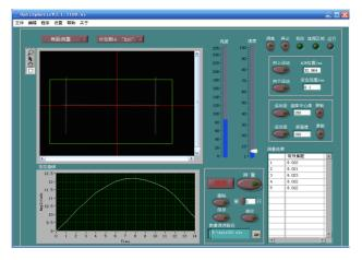
is used to test the eccentricity, and a parallel light is conducted to the lens, and either pass through (transmission mode) or reflected (reflection mode) by the lens, and generate an image on the detector. The software would trace an image change while the lens is rotated. The eccentricity is calculated based on the circle radius of the rotation image.
