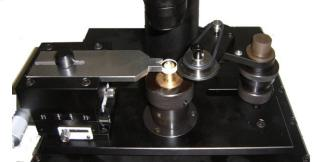
wheel is run by the precision motor to drive the tested lens rotated automatically, then software record rotation image and show on the eccentricity data either in um or arc-min.
