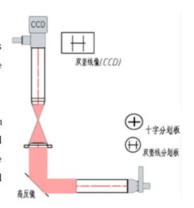
The contration is also an importance for the lens to imaging. According to ISO 10110 the eccentricity is present when the optical and the reference axis of a lens do not coincide, respectively these are different in position or direction. The cross reticle
